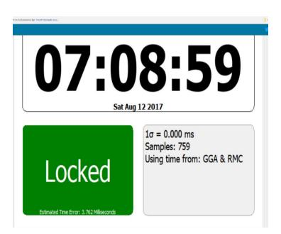
With this program running, the longer it is in operation the more accurate the time. As you can see above this has taken 759 samples and the difference between the PC Clock and the GPS Time is 3.762 Milliseconds. That number will become smaller the longer the program runs. Which will equate to the "DT" time on your WSJT/FT8 Software to be at or close to 0.0. Yes it will fluctuate some but statistically more accurate and more stable.
