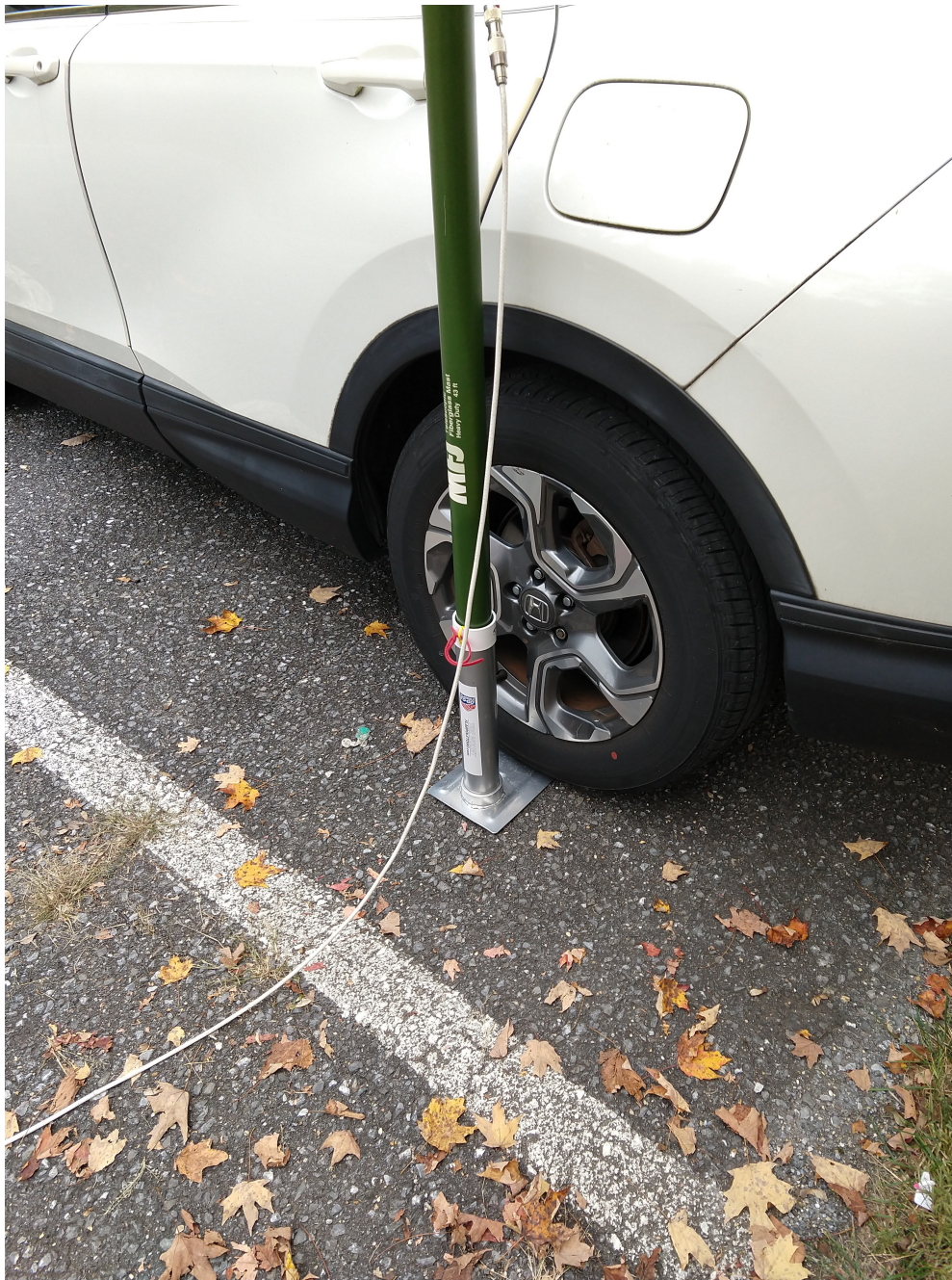
flagpole tire mount – driver mirror aimed down
