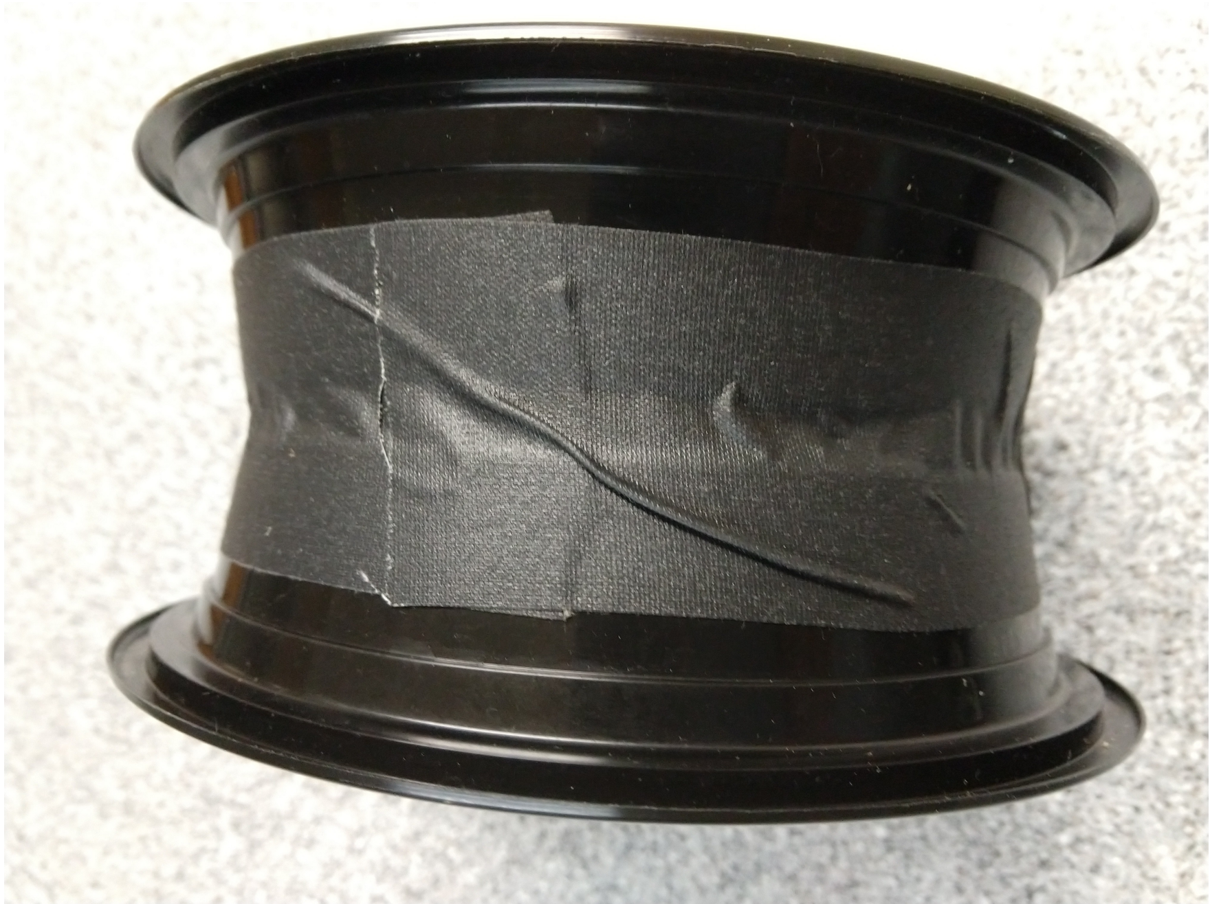
bobbin made from two shallow carry-out food containers
