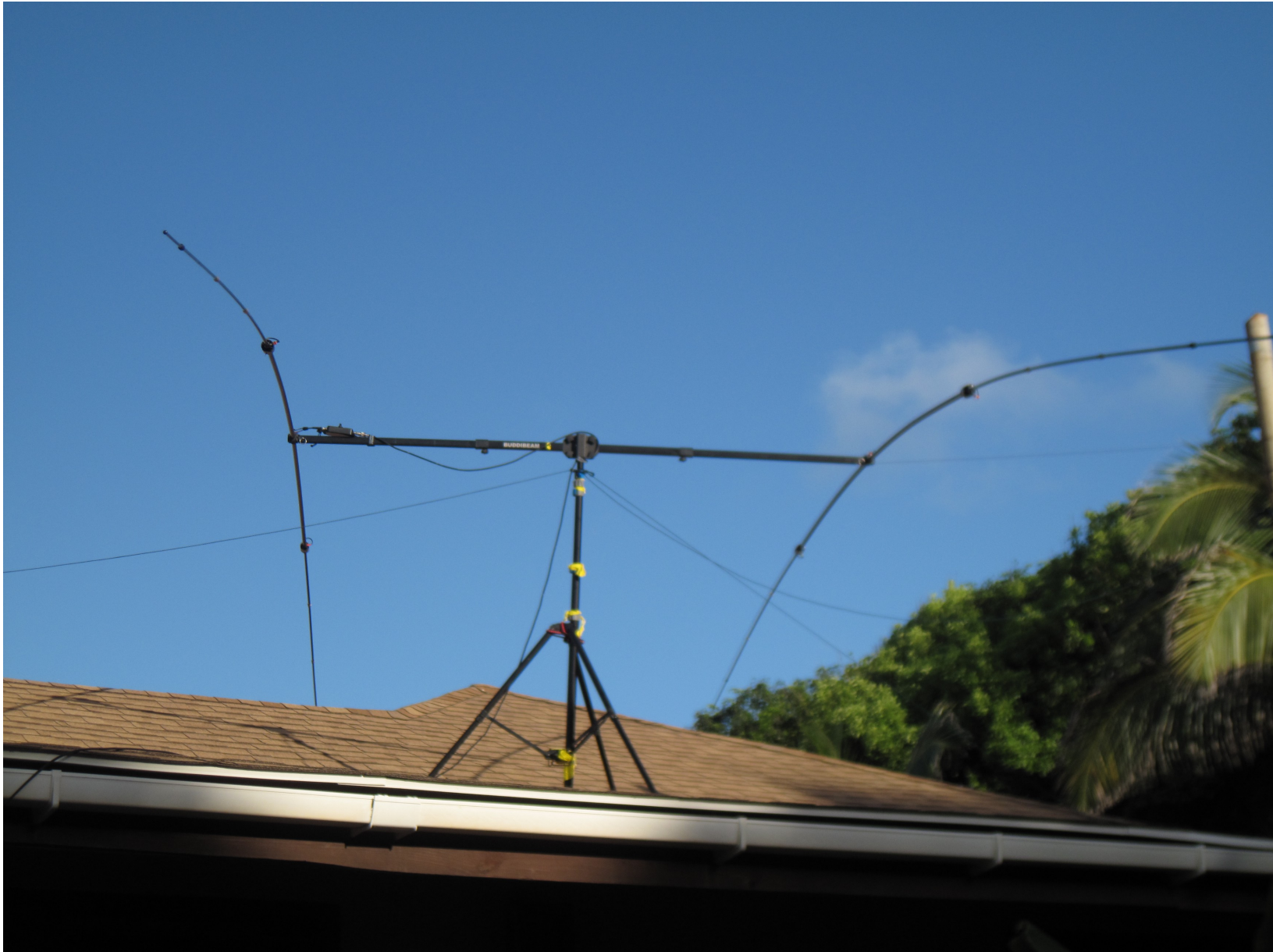
2 element 20 m Yagi on roof
